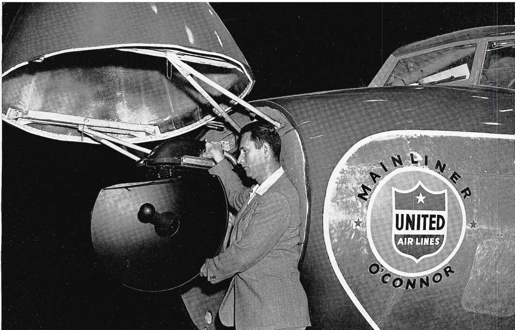
L. E. Sebald, project engineer at the San Francisco maintenance base of United Air Lines, demonstrates antenna of RCA C-band radar on "Mainliner O'Connor." It is the first installation in a $4,000,000 program to equip the company's entire fleet with the new weather-mapping device. Nose of the Convair 340 has been extended 28½ inches to house radar antenna and gear mechanism.
