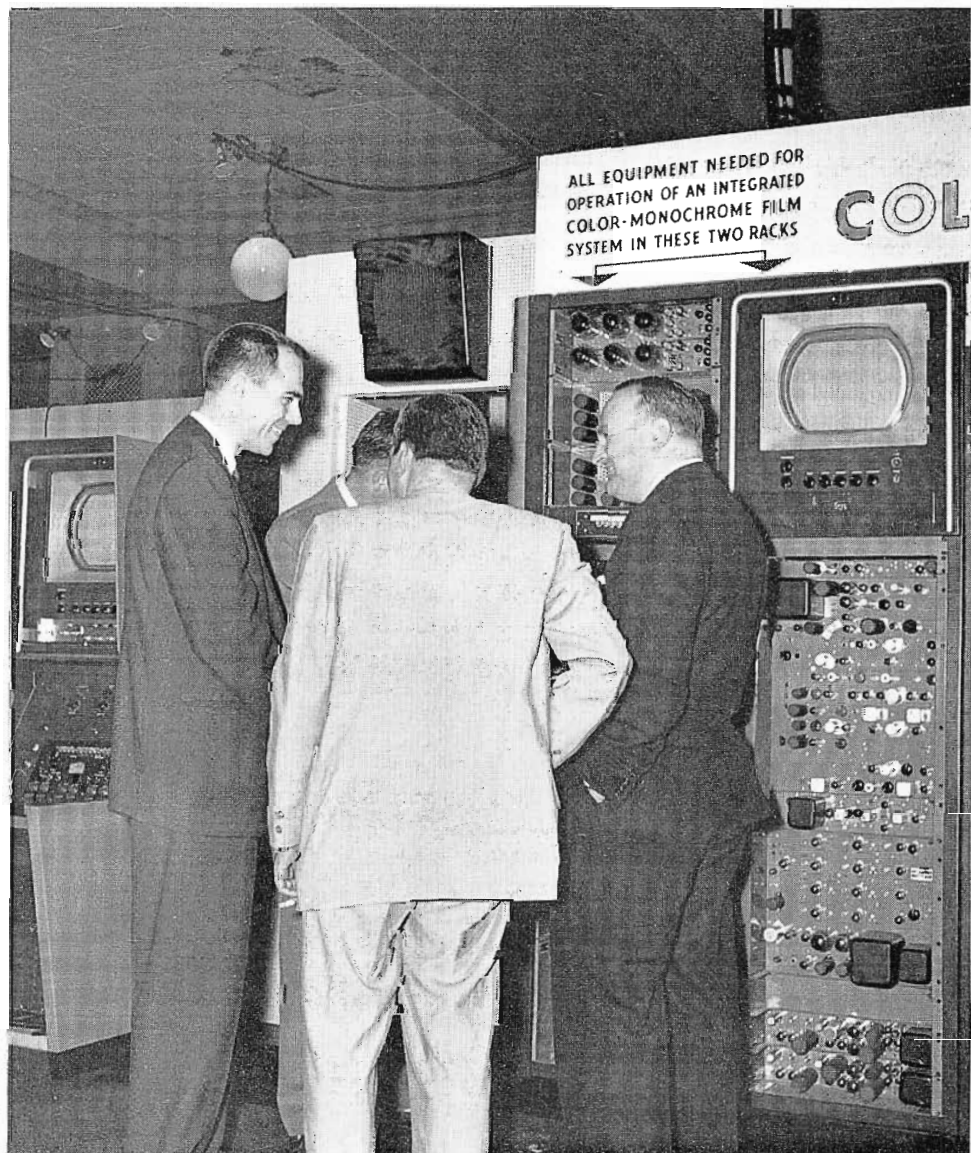
FIG. 8. Complete auxiliary equipment for RCA color-monochrome film system is housed in two cabinet racks.
